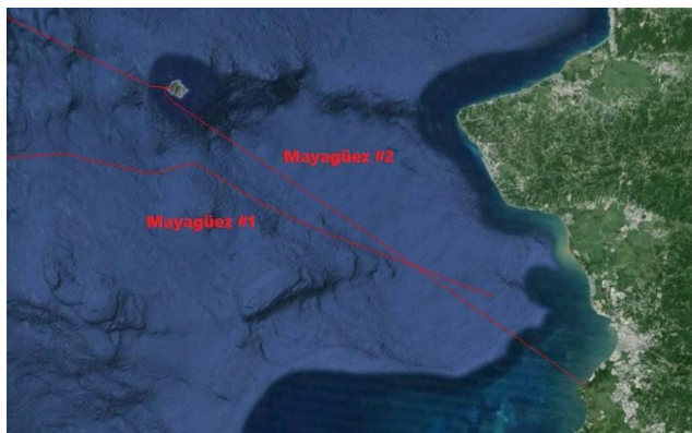
Fig.2 SAJ-2015-02643 (SP-DCM) known as Mayagüez #1 (Mayagüez-Santo Domingo) and SAJ-2015-02641 (SP-DCM) known as Mayagüez #2 (Mayagüez-Desecheo and Desecheo-Dominican Republic), are out of service telegraph submarine cables coming out from the west coast of Mayagüez, Puerto Rico.
