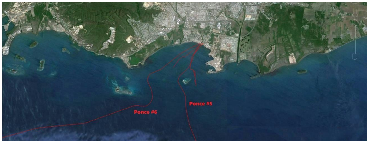
Fig.4 SAJ-2015-02640 (SP-DCM) known as Ponce #5 (Ponce-St. Croix) and SAJ-2015-02639 (SP-DCM) known as Ponce #6 (Ponce-Jamaica), are out of service telegraph submarine cables coming out from the south coast of Ponce, Puerto Rico.
